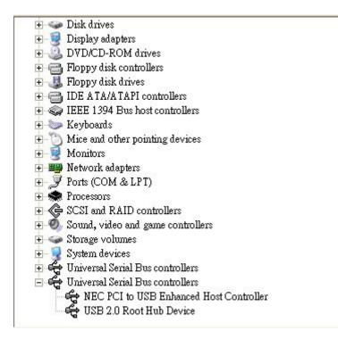
Note! If there is a yellow exclamation mark on "NEC PCI to USB 2.0 Enhanced Host Controller" or "USB 2.0 Root Hub Device", please remove this item from the "Device Manager" by clicking the "Uninstall" button and click "Refresh" to re-install this driver again.
